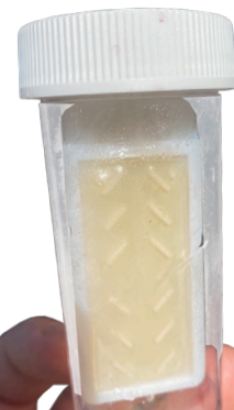
Bacteria dip slide tests results continue to show bacterial levels at 10^0 indicating excellent control of bacteria in the cooling tower system.
