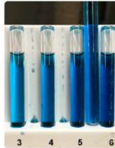
Before - Dissolved oxygen test results 5-6ppm.
