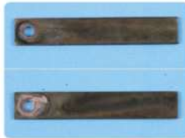
Corrosion coupons lost only .0692 mils/yr, which is beyond EXCELLENT according to the chart on the next page!
