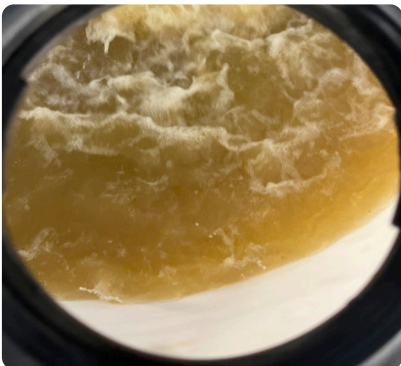
A view of the dirty water in the backwash tank from the CTF sub-micron filter
