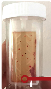
Prior to treatment , the water was very dirty and lab results from March 17th, 2023 indicated a high 10^3 bacteria count
