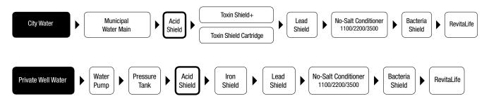
If a lawn or garden irrigation system or open loop heating/cooling system is to be treated, a separate Acid Shield will be necessary. Contact EasyWater Tech Support for more information on these installations.
