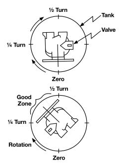
Note: Do <u>NOT</u> use the drain connector to tighten the valve on the tank. This can break the drain connection or crack the valve.
